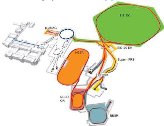
Figure 1: Existing GSI (left) and future FAIR accelerator complex (NESR, RESR not part of the start version).
