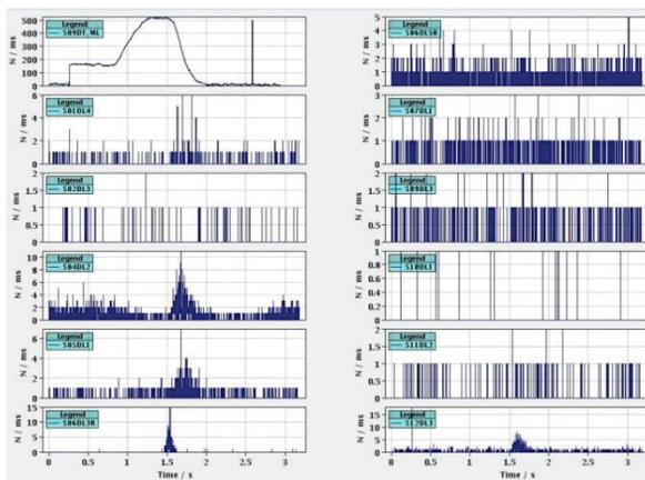
Figure 4: Screenshot of the LASSIE system at GSI SIS18. Top left: signal of dc current transformer; 11 beam loss monitors around the synchrotron.
