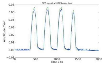
Figure 3: Raw FCT signal (blue) and values corrected for cable response (green).
