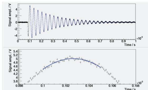
Figure 2: Top: raw RT signal (black) and fit curve (blue); Bottom: first maximum (black) and 2<sup>nd</sup> order polynomial fit (blue).
