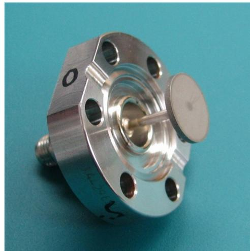
Figure 1: A photograph of the button electrode.
