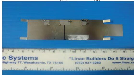
Figure 1: Picture of the shim holder with magnetic shims on it.
