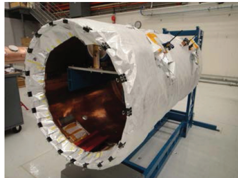
Figure 4: 60-K radiation shield with MLI blankets.
