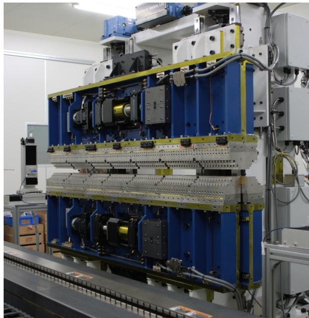
Figure 1: New QP-APPLE-II undulator on the magnetic measurement bench.
