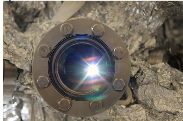
Figure 7: Observed synchrotron radiation light from the QP-APPLE-II undulator.
