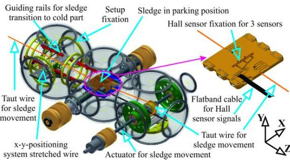
Figure 2: Schematic drawing of the local field measurements setup.
