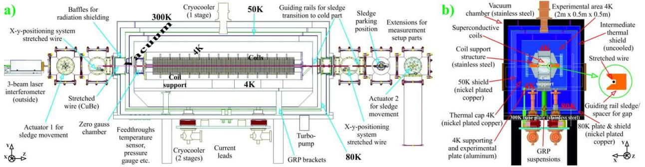
Figure 1: Side view (a) and sectional view along z-axis (b) of CASPER II showing the different temperature regions and the equipment for local and integral field measurements.
