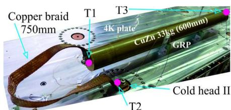
Figure 5: Picture of the 4 K plate with the test setup for the final acceptance test.
