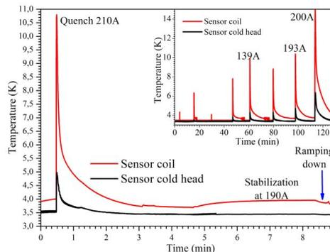
Figure 7: Temperatures over time during quench tests at selected measurement points.
