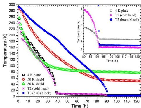
Figure 6: Graph with time dependence of selected temperatures during final acceptance test.
