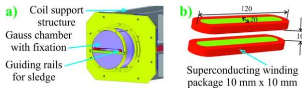
Figure 3: Planned components to check Hall sample calibration: a) zero Gauss chamber, b) racetrack coils.
