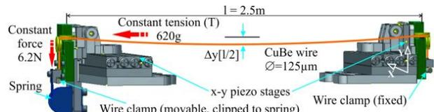
Figure 4: Sketch of the stretched wire setup.
