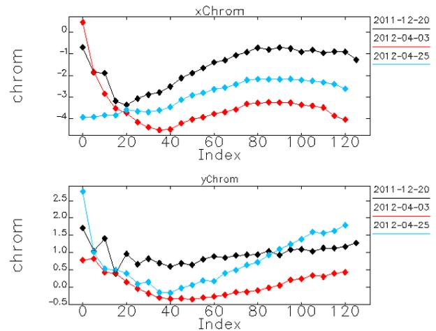
Figure 5: Plot of x- and y-chromaticity of booster low-emittance lattice during tuning processes. The data for optimized result are in blue color.
