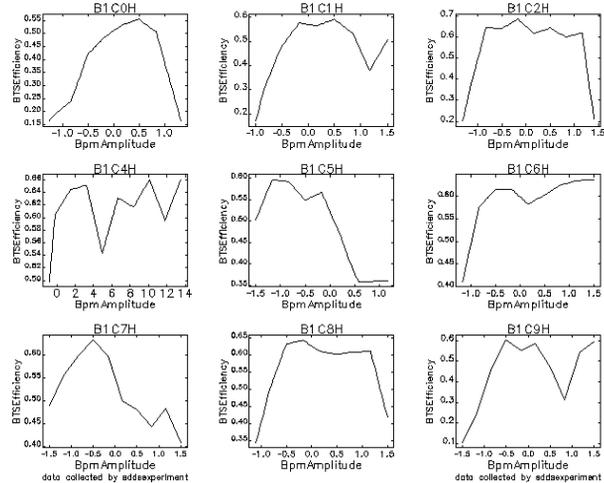
Figure 3: Plot of the bump scan data. The y-axis is PTB-to-BTS efficiency while the x-axis is the the corrector bump amplitude.
