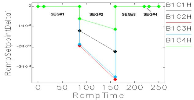
Figure 2: Plot of ramp setpoint changes of the four correctors of the B1C2H bump. The tuning segments are: 12-86 ms, 86-160 ms, 160-220 ms, and 220-230 ms.
