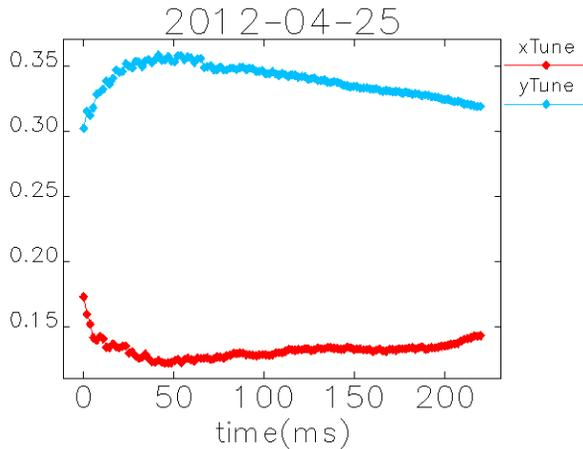
Figure 1: Plots of x- and y-tune of low-emittance lattice after optimization.
