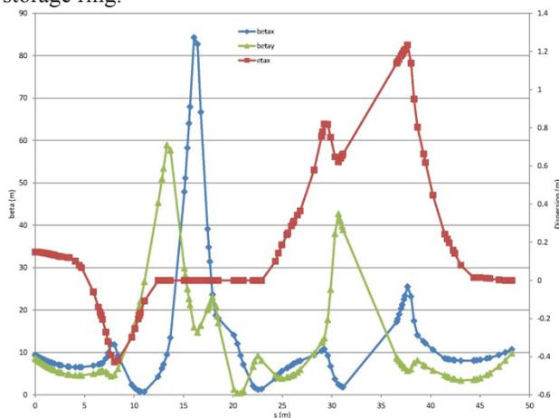
Figure 7: Beta and Dispersion functions of the Booster to Storage Ring Transfer line for Storage Ring injection.
