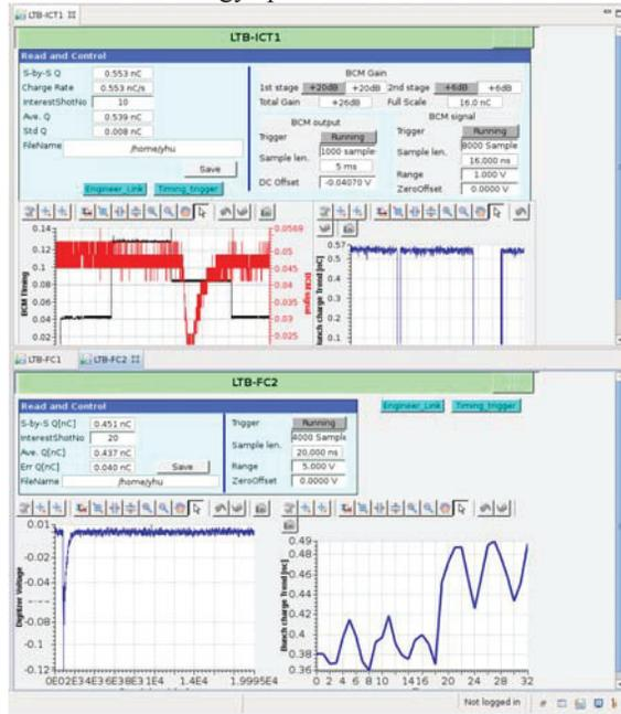
Figure 3: Comparison of the integrating current transformer and a beam dump faraday cup in the transport line.
