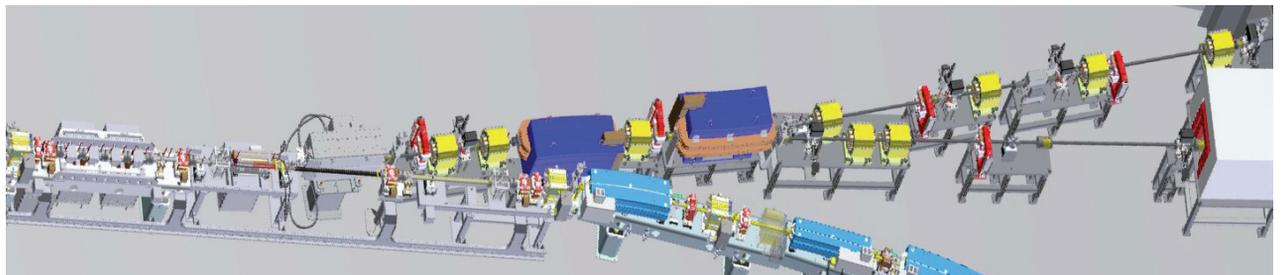
Figure 5: Booster to Storage Ring Transport Line Part I, showing booster extraction, the beam dump line and the injection path to the storage ring.
