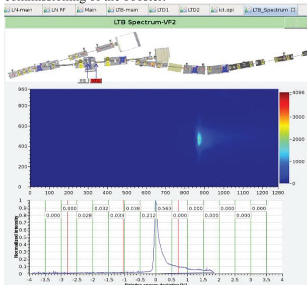
Figure 2: Screenshot of beam on the YAG screen at LB-VF2 in the spectrometer arm.
