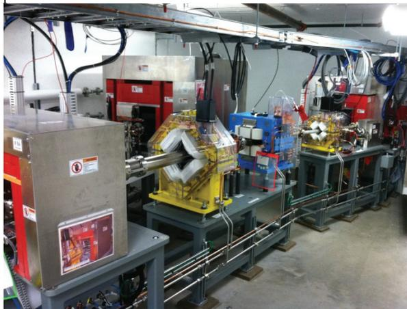
Figure 1: LtB part I installation. Spectrometer beamline shown. Energy Slit in the foreground, beam dumps in the background.
