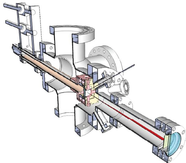
Figure 1: System for measuring cathode transverse momentum.
