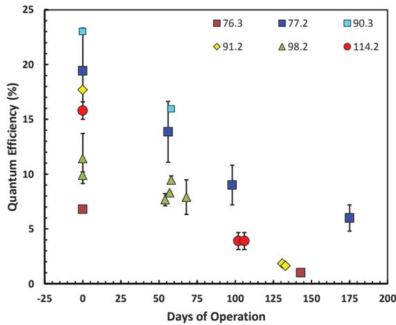
Figure 1: Operational lifetime of cathodes used at FLASH from 2009 to 2012. The legend shows the cathode ID.
