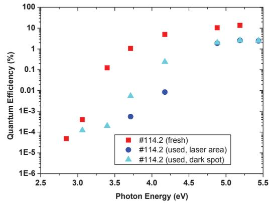
Figure 6: Spectral response of cathode 114.2. The response of the fresh cathode is compared with the "black spot" and the area, where the laser beam hit the cathode. Remarkable is the reduction of QE for lower photon energies.
