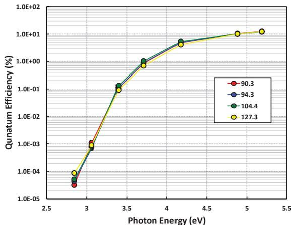
Figure 2: Spectral response of four recently produced  $\text{Cs}_2\text{Te}$  cathodes. Within the measurement error, the spectral response of all cathodes is equal.
