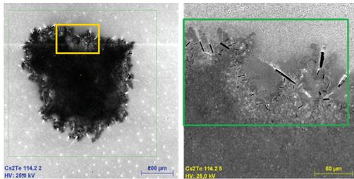
Figure 4: (Left) SEM image of the "black spot" of Fig. 3. The scale (lower left blue bar) is 200 μm. (Right) Magnification of the area shown by a yellow rectangle (scale 60 μm).
