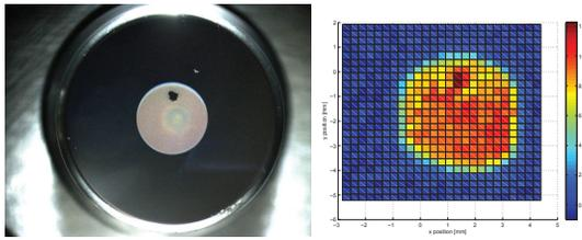
Figure 3: (Left) Cathode 114.2 showing a "black spot". The spot with a dimension of about 0.5 mm appeared during operation in the RF gun at FLASH. In addition, discoloration is visible where the laser beam has hit the cathode. The tiny white spot above the cathode is a particle. (Right) A QE-map of the cathode. The "black spot" on the left picture has a higher QE than the average. The color code scale is the measured charge in pC.
