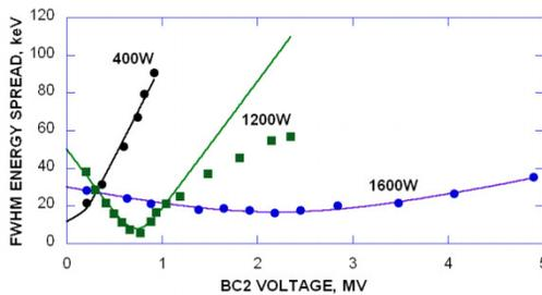
Figure 7: FWHM energy spread as a function of the BC2 voltage. The BC2 phase is set to zero-cross.
