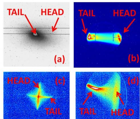
Figure 5: Beam images on screens: (a) screen YAG-02, horizontal lines show the position of beam profiles showed in Fig.2,a; (b) screen YAG-05 in dispersive region; (c) screen YAG-04 at  $P_b=1.0\text{kW}$ ; (d) the same but BC2 is set to zero-cross.
