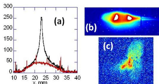
Figure 2: (a) beam single pixel profiles; black – through the centre of the beam image on YAG-02 screen, red – with offset from the centre; (b) beam image in the dispersive section, on YAG-05 screen; (c) beam image on a post linac OTR screen.
