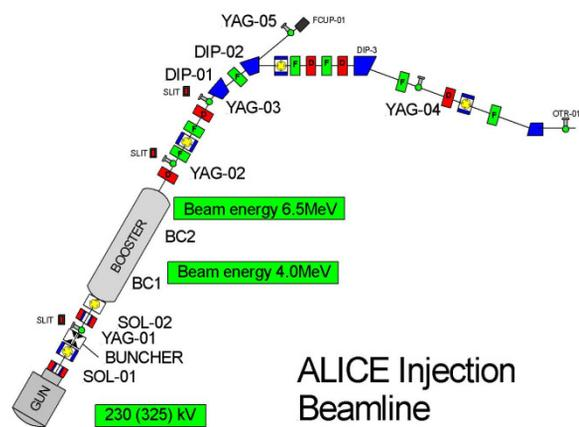
Figure 1: Layout of the ALICE injection line.
