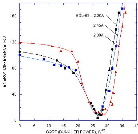
Figure 3: Energy difference between two peaks in the beam energy spectra as a function of the buncher power and the solenoid field. BC2 phase here is set to +40deg.
