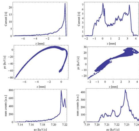
Figure 8: Simulated (ASTRA) longitudinal bunch profile (top), longitudinal phase space (middle) and energy spectra (bottom) at buncher powers of 400W (left column) and 1100W (right column). Gun voltage 230kV.
