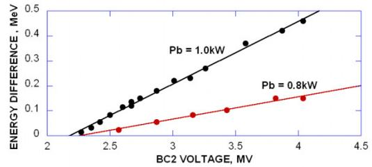
Figure 4: Energy difference between two peaks in the beam energy spectra as a function of the BC2 voltage. The BC2 phase is set to zero-cross.
