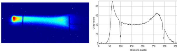
Figure 6: “Two beam” structure on YAG-05 screen at significantly reduced buncher power of 0.4kW.
