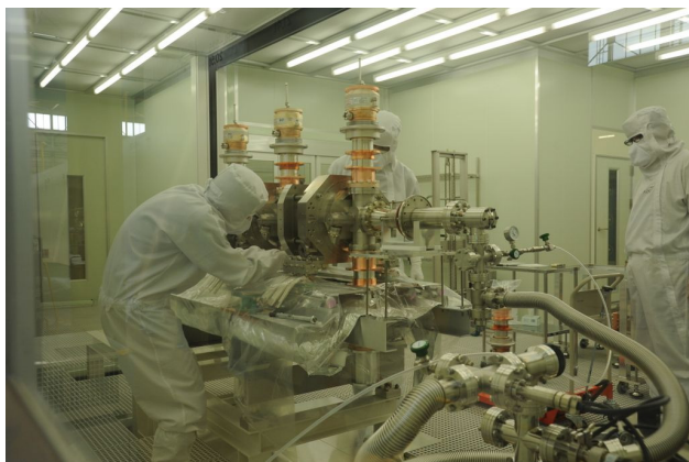
Figure 5: Assembly of a string of injector cavities at KEK.
