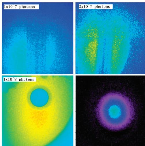
Figure 5: X-ray images with different integrated X-ray flux. The bottom-right image was the image for a three layer ball. The integrated x-ray flux is about  $6 \times 10^7$  photons.
