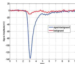
Figure 2: typical X-ray signal and background from the MCP detector.
