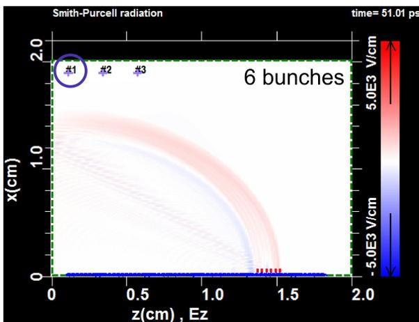
Figure 1: “Screen shot” of the simulated CSPR generation process. The radiation was generated by 6 bunches (shown as the red dots) and was measured at the numbered points.
