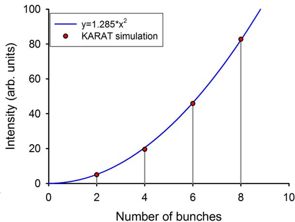
Figure 3: Dependence of the main spectral peak maximum on the number of bunches
