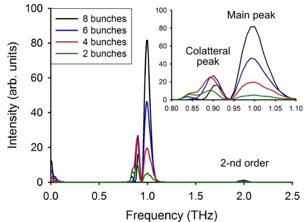
Figure 2: CSPR power spectrum for the different number of bunches in the train measured at the point #1. The insert shows the radiation in the neighborhood of 1 THz frequency in more details
