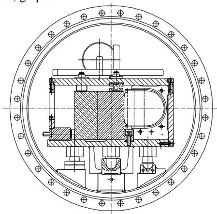
Figure 3: Cross section of the TCDQ structure showing the graphite (left) and CFC (right) absorber blocks.
