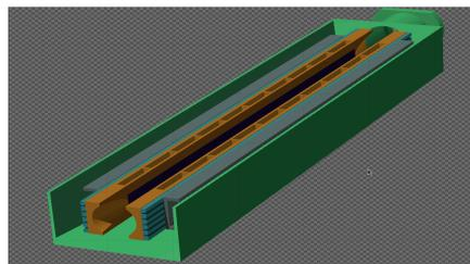
Figure 1: FLUKA model of the TCT. The tungsten-based insert can be seen on the internal jaw surface.
