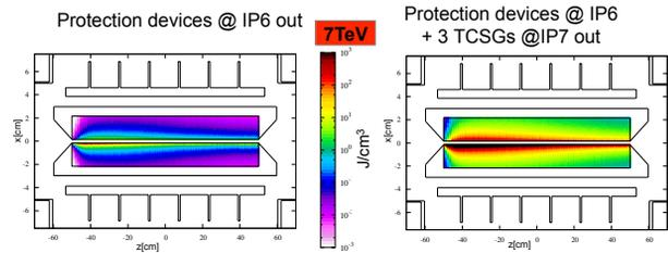
Figure 5: 2D energy deposition maps cut at the beam height due by 7TeV impacting protons. The two insert maps are superimposed to the jaw geometry cut. The binning used to score is 0.01x0.01x0.5 cm3. In the picture an average over 4 bins in the vertical direction is shown.
