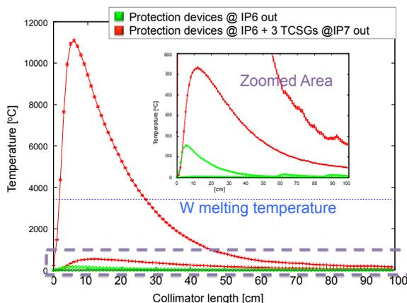
Figure 4: Temperature peak profiles of the two TCT jaws for each different accident layout at 7TeV. As can be seen, the jaws are asymmetrically loaded. Statistic errors are less than 5% for peak values.
