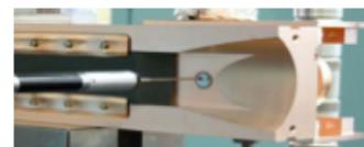
Figure 6: BPM button integrated on the tapering part at the end of a collimator jaw.
