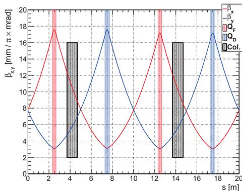
Figure 2: Two periods of the studied FODO channel with transverse  $\beta$  functions, quadrupole magnets, and possible location of collimators.
