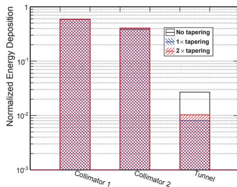
Figure 3: The relative distribution of energy deposition in the test beamline.
