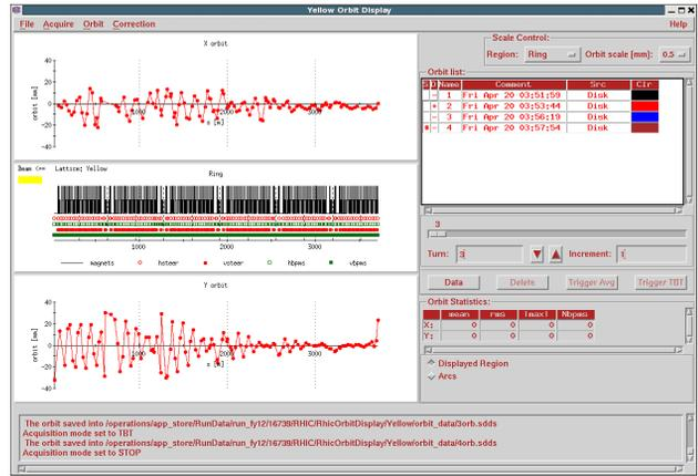
Figure 6: Measured orbit after putting in one round of correction using new steering algorithm, beam survived one turn
