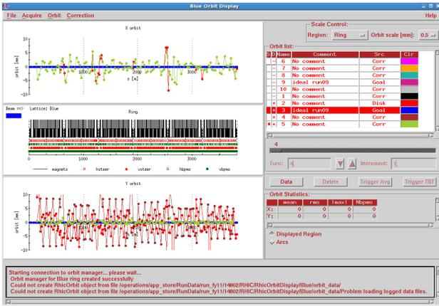
Figure 4: Test of new steering algorithms in blue vertical plane: in the lower plot, red is the first turn of a saved injection orbit, cyan is the predicted orbit after correction, horizontal orbit in the upper plot stays untouched
