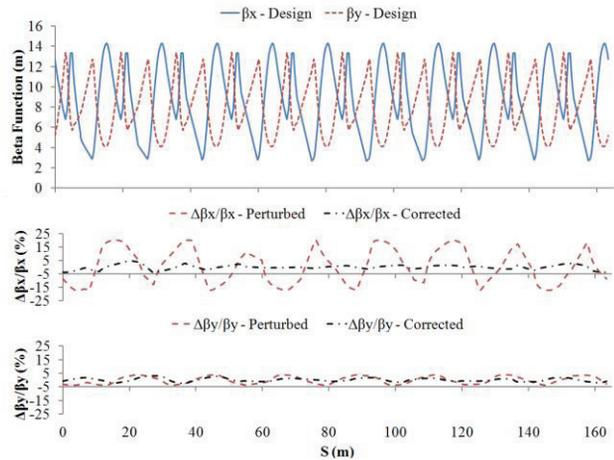
Figure 8: Betatron function for the ISIS synchrotron (top) and perturbation to this function with and without corrections for horizontal (middle) and vertical (bottom) planes.
