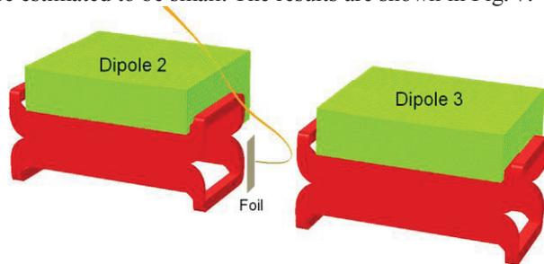
Figure 7: Electron trajectories in injection dipole fringe fields.
