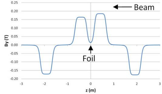
Figure 5: Longitudinal profile of the vertical magnetic field,  $B_y$ , along  $x=y=0$  axis through the injection region.
