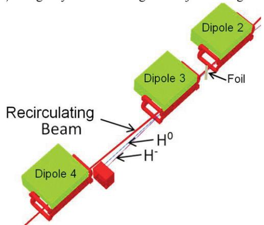
Figure 6: Beams tracked through a 180 MeV injection region.
