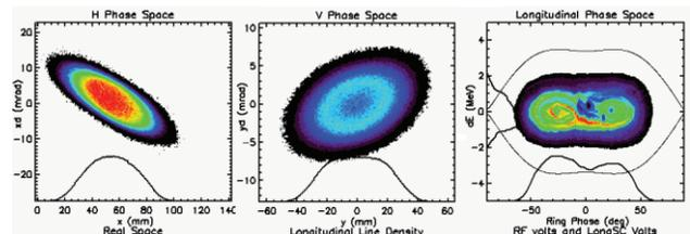
Figure 2: Transverse and longitudinal beam distributions at the end of injection, from 3D ORBIT simulations.
