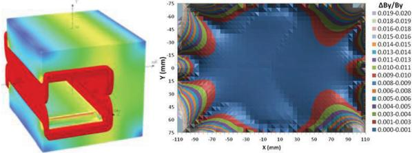
Figure 3: 180 MeV injection dipole model (left) and field homogeneity,  $\Delta B_y/B_y$  (right).
