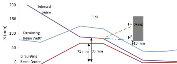
Figure 4: Geometric design trajectories for a 180 MeV injection system.
