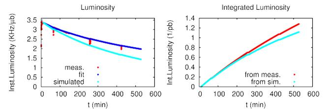
Figure 7: On the left, the instantaneous luminosity actually measured on October 16 by CMS is shown (red) together with the luminosity obtained after applying the largest reduction observed during the October 13 experiment (cyan). The corresponding integrals are shown on the right.
