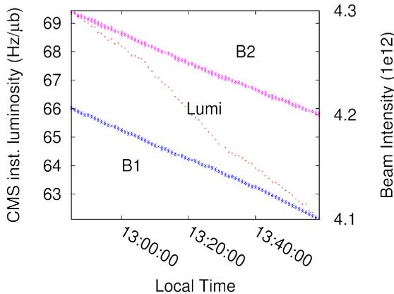
Figure 2: Luminosity vs. time (red) shows a kink at about 13h10 corresponding to the moment B1 and B2 cleaning is switched on. The second kink at about 13h34 corresponds to the moment the cleaning is turned off. The BCT (blue for B1, magenta for B2) does not show kinks.
