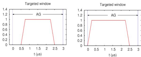
Figure 4: “Short” (left) and “long” (right) kicker pulse.
