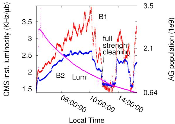
Figure 5: CMS luminosity (magenta), B1 (red) and B2 (blue) AG population during October 13 experiment. The luminosity run started around 3h00, AG cleaning (with various settings) at 10h17.
