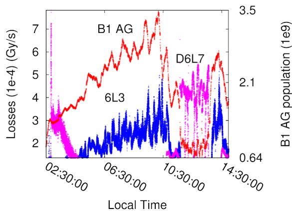
Figure 6: B1 AG population (red), losses at betatron collimator TCP.D6L7.B1 (magenta) and momentum collimator TCP.6L3.B1 (blue).
