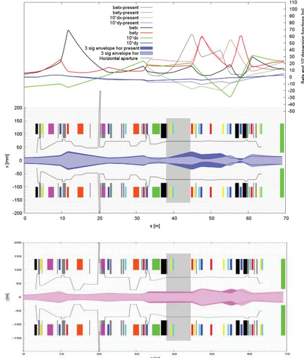
Figure 4: The top part of the plot shows the TL optics matched to existing PS injection parameters. In the lower part the horizontal (blue) and vertical (pink)  $3\sigma$  LHC beam sizes are plotted for the present (dark) and upgrade (light) situation.
