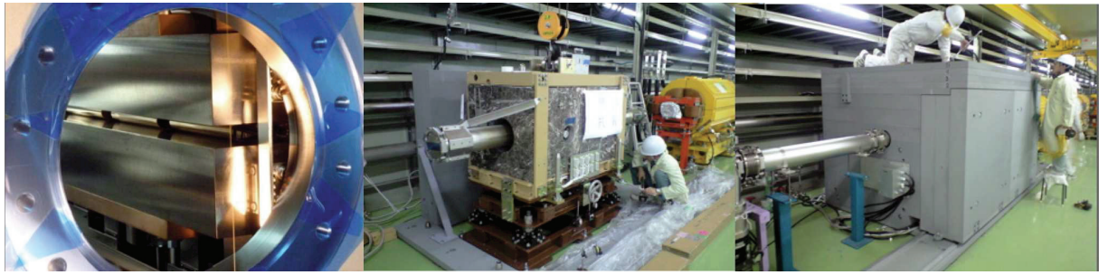
Figure 2: Photographs of the collimator for the slow extraction.
