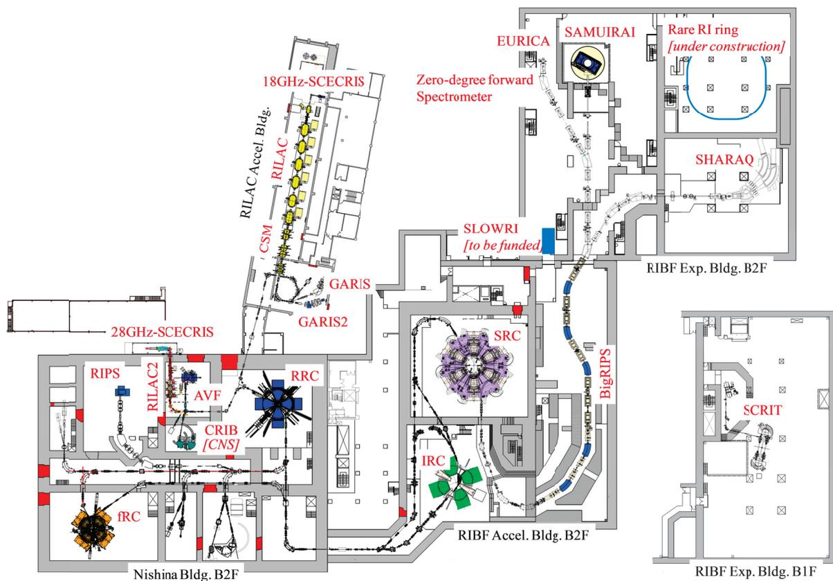
Figure 1: RIBF layout. Three types of injectors and four ring cyclotrons.
