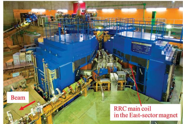
Figure 2: RRC overview. The main coil of the East-sector magnet will be replaced with a newly fabricated coil in the summer of 2012.
