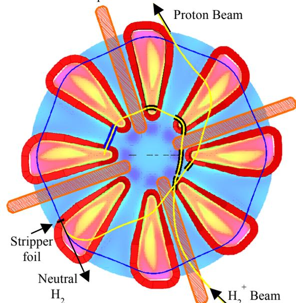
Figure 1: DSRC Layout, with the injection and extraction trajectory. Coils and cavities are also shown.
