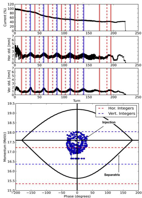
Figure 2: Similar to Fig. 1 but with injection near to the SFP, crossing speed  $Q' \approx 0.09$ . No net amplitude growth is evident.
