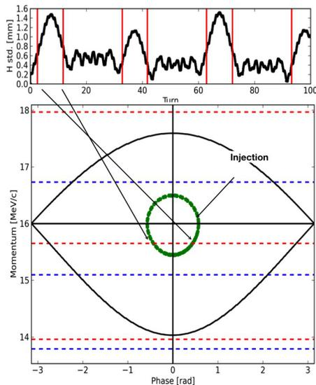
Figure 4: Acceleration of a single particle in a PyZgoubi model of EMMA, the particle injected close to the SFP such that the crossing rate is larger than in Fig. 3. Acceleration voltage was 0.2 MV/turn, crossing rate  $Q' = 0.09$ .
