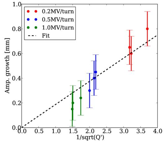
Figure 5: Amplitude growth as a function of crossing speed in a single particle simulation.
