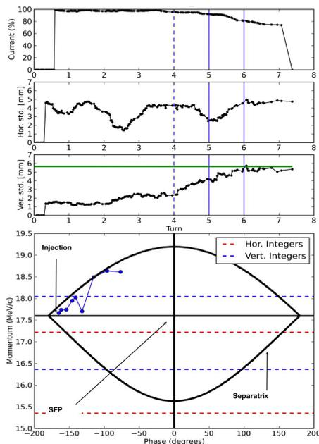
Figure 1: Amplitude growth and longitudinal phase space for a bunch accelerated at 0.2 MV/turn and crossing speeds of  $Q' \approx 0.07$ . Red/blue indicate horizontal/vertical integer tunes. Similar behaviour is seen at other accelerating voltages.
