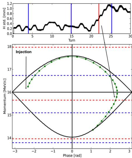
Figure 3: Acceleration of a single particle in a PyZgoubi model of EMMA, the particle injected near to the separatrix such that the crossing rate is small. Amplitude growth is derived from the standard deviation of oscillations before and after times corresponding to the width of the horizontal integer tune (shown in red, vertical integer tunes shown in blue). Acceleration voltage was 0.2 MV/turn, crossing rate  $Q' = 0.07$ .
