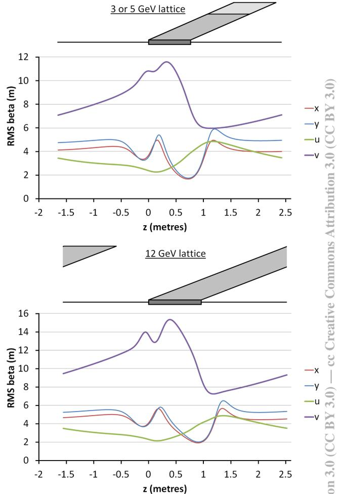
Figure 4: Beta functions in the two lattices, in non-skew and skew coordinates. Magnet size is to scale in  $z$  and  $y$ .
