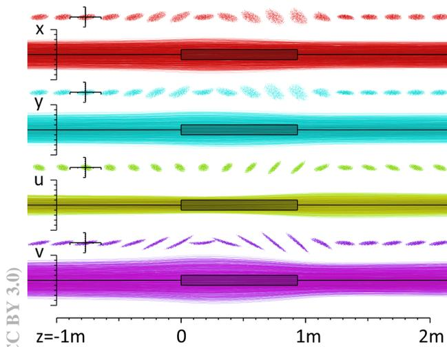
Figure 5: Phase space and beam evolution through the 12 GeV ring cell at injection energy. Transverse scale is  $\pm 5$  cm and  $x', y', u', v'$  ranges are  $\pm 20$  mrad.
