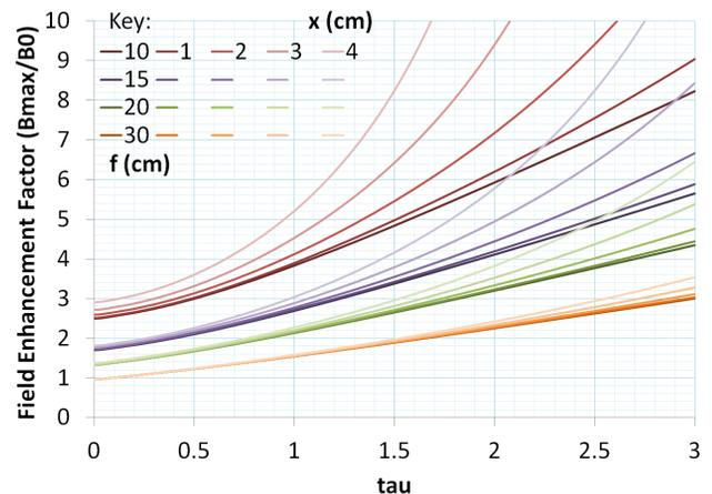
Figure 2: Field enhancements as a function of  $\tau$ , fringe length ( $f$ ) and distance from mid-plane ( $x$ ) from 0 to 4 cm, in the 3 or 5 GeV magnet design with  $k = 2.05 \text{ m}^{-1}$ .
