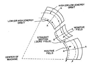
Figure 1: Schematic figure of a radial-sector FFAG [6]). As the beam is accelerated, the orbit moves to outside.
