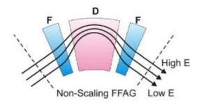
Figure 3: Orbits of a non-scaling FFAG are compressed within a short dimension [9].
