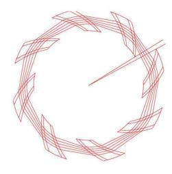
Figure 2: Spiral-sector FFAG and its orbits [7]. Again, the beam orbit moves outside, as it is accelerated.
