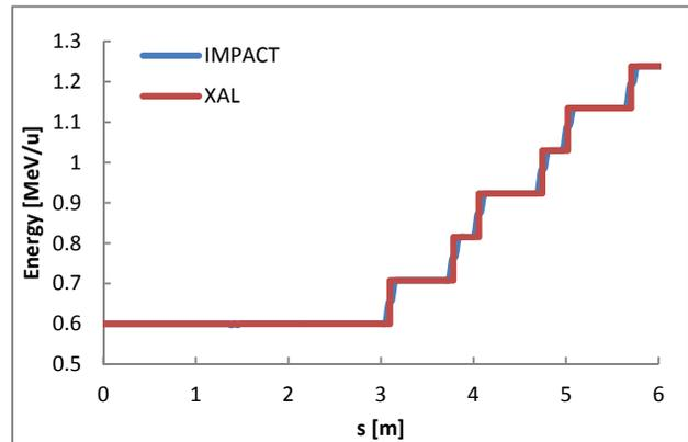
Figure 4: ReA3 Linac through second cryomodule Energy [MeV/u] in XAL and IMPACT.
