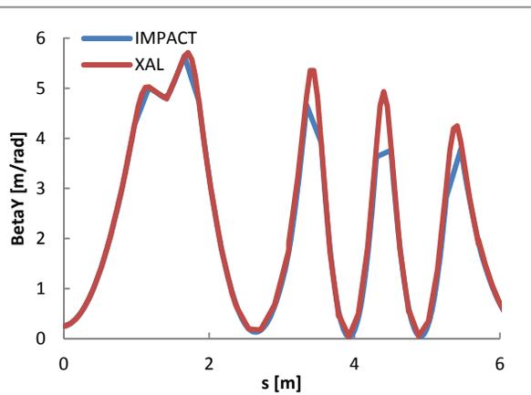
Figure 6: ReA3 Linac through second cryomodule BetaY [m/rad] in XAL and IMPACT.
