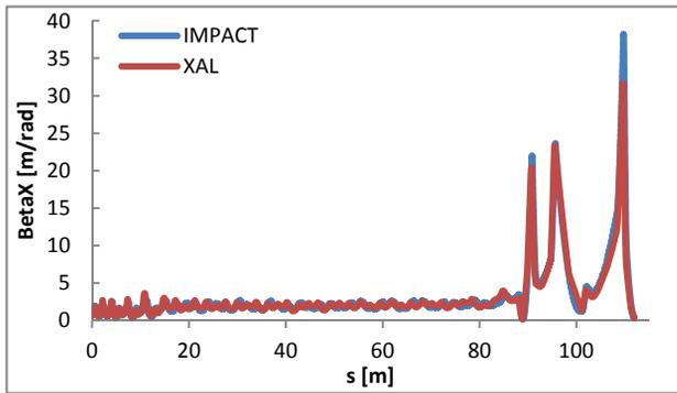
Figure 5: Current design FRIB Segment 1 through first bending section BetaX [m/rad] in XAL and IMPACT.
