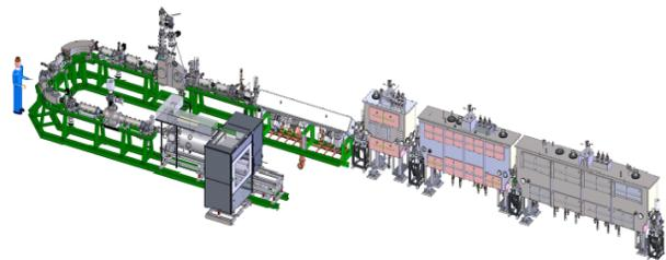
Figure 1: ReA3 Layout, including EBIT charge breeder, Q/A section, RFQ and Linac.
