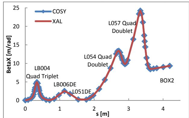
Figure 3: LB to BOX2 BetaX in XAL and COSY. In all data plots, s refers to the ideal particle path length.
