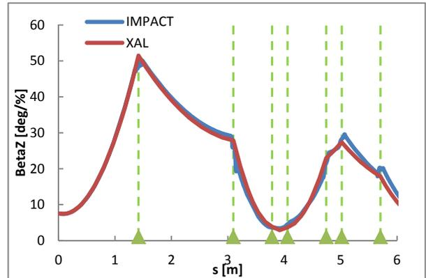
Figure 7: ReA3 Linac through second cryomodule BetaZ [deg/%] in XAL and IMPACT.
