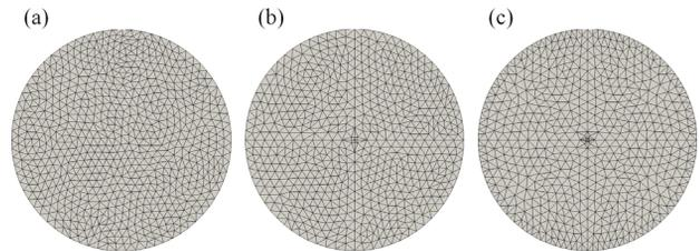
Figure 7: Cross section of a tetrahedral mesh in a plane normal to the longitudinal axis of the resonator for an arbitrary unstructured mesh (a), a mesh aligned at the coordinate planes (b) and a true symmetric mesh (c) [4].
