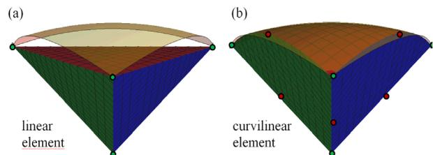
Figure 4: Linear versus curvilinear tetrahedral element [4].
