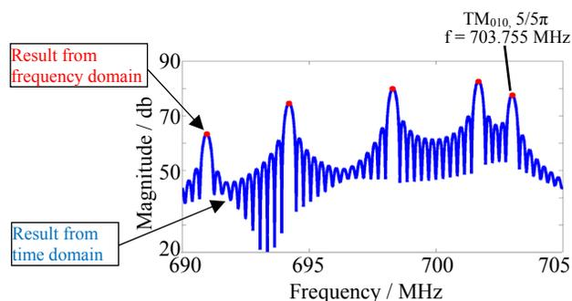
Figure 2: Eigenmode spectrum of  $TM_{010}$  passband.
