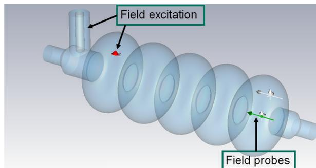
Figure 1: Power coupler and discrete port in cell 1, Field detection in cell 5.
