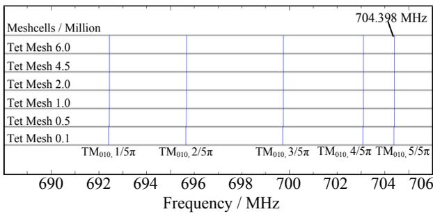
Figure 5: Convergence analysis of various numbers of tetrahedral elements based on the resonance frequency of the fundamental modes ( $TM_{010}$ ) in a SPL cavity.
