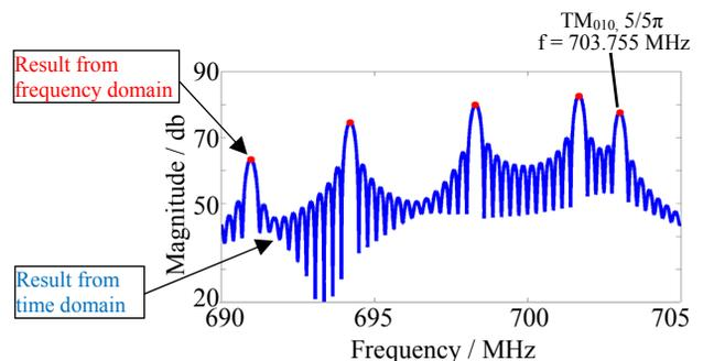
Figure 2: Eigenmode spectrum of  $TM_{010}$  passband.
