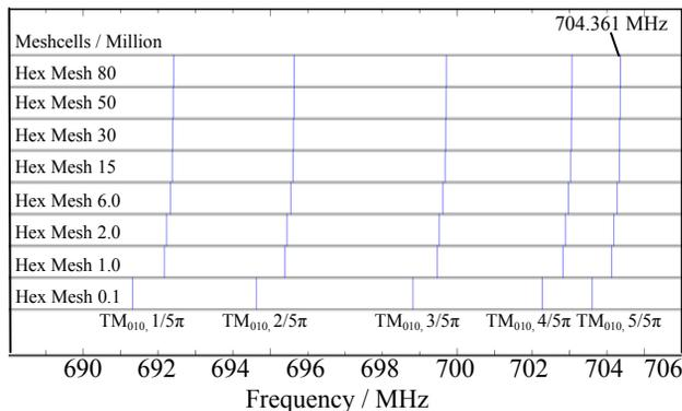
Figure 3: Convergence analysis of various numbers of hexahedral elements based on the resonance frequency of the fundamental modes (TM<sub>010</sub>) in a SPL cavity.
