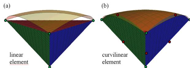
Figure 4: Linear versus curvilinear tetrahedral element [4].
