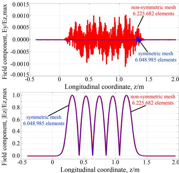
Figure 6: Evaluation of the electric field strength along the cavity axis. All Cartesian components are normalized to the maximum longitudinal field value  $E_{z,max}$ . All calculations are performed using non-symmetrical and symmetrical curvilinear tetrahedral elements.
