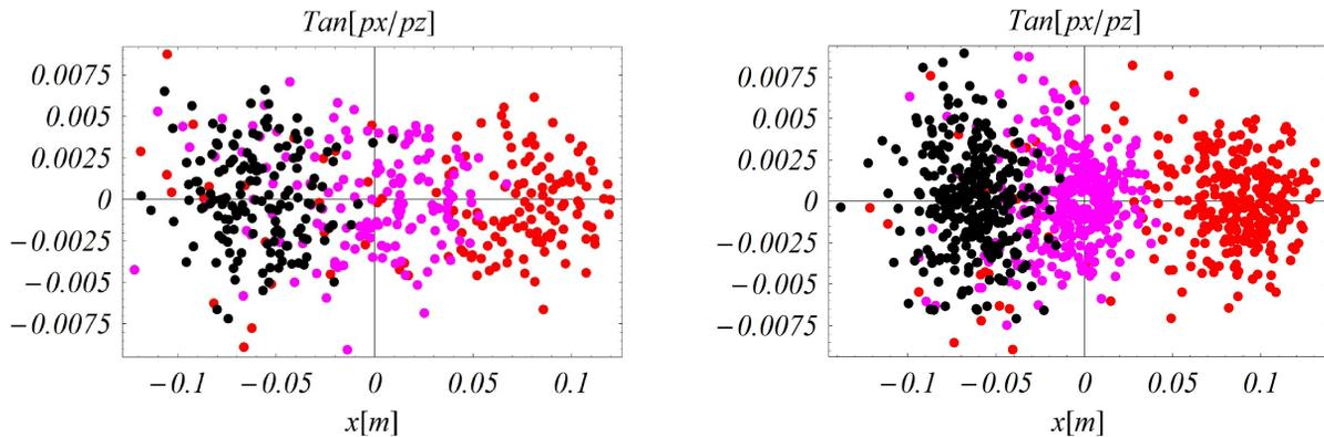
Figure 4: Horizontal phase space during acceleration before (left) and after (right) adjusting initial conditions to take into account the non-parabolic energy dependence in the time of flight. Colors are black for the initial distribution, pink at an intermediate energy, and red at the final energy. The large density after the adjustment demonstrates our improved transmission. The horizontal position of the beam becomes more positive with increasing energy.
