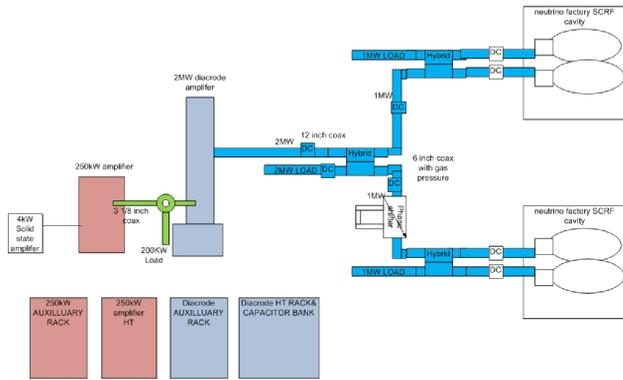
Figure 5: RF power source and distribution schematic.
