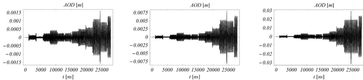
Figure 2: Orbit distortion (in m) during acceleration for septum fields of (left to right) 1.8 T, 2.2 T, and 2.6 T.
