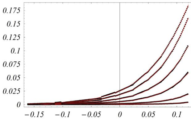
Figure 1: Septum stray field (in T) as a function of horizontal position (in m). Curves are for a main septum field of (bottom to top) 1.8 T, 2.2 T, 2.6 T, 3.1 T, 3.5 T, and 3.9 T.
