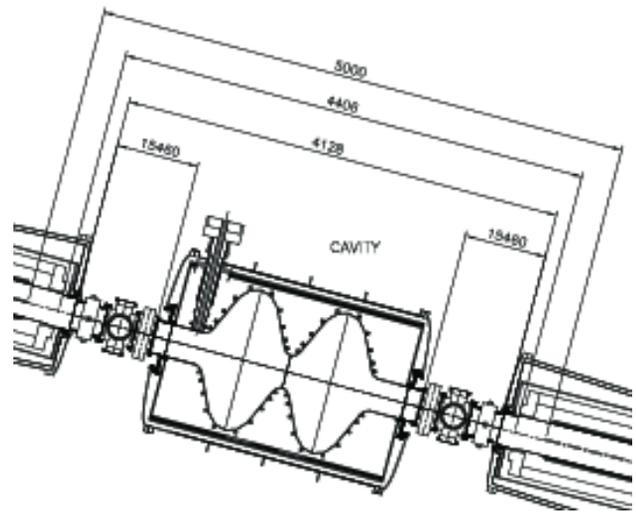
Figure 3: Drawing showing the RF cavity between two triplet cells, all with their cryostats. Dimensions are in mm.
