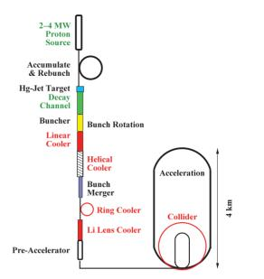
Figure 4: Schematic of a 1.5-TeV muon collider.
