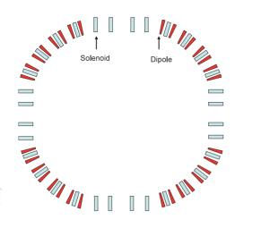
Figure 7: Schematic drawing of a four-sided ring using dipoles-solenoids for muon 6D cooling. The ring cooler 6D system is fully described in Reference 3.
