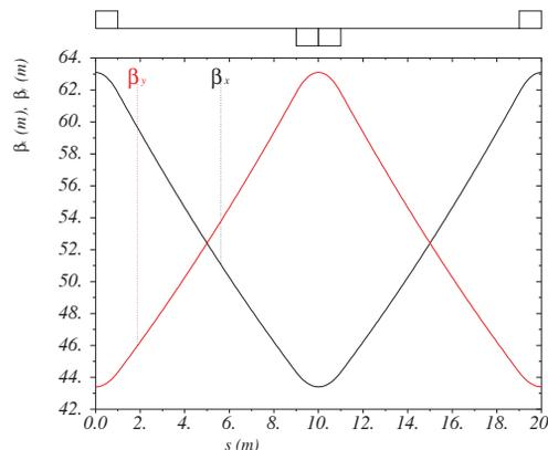
Figure 1: Optics in one production straight cell.
