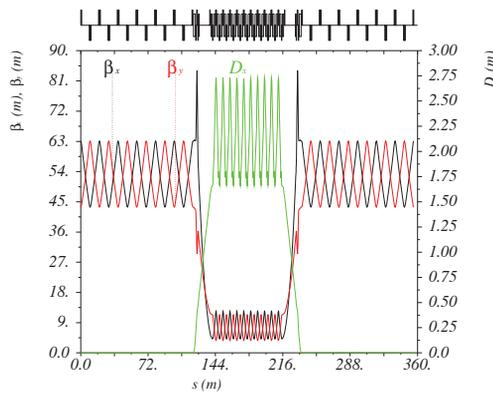
Figure 2: Optics over half a ring for a preliminary 10 GeV design. The horizontal axis extends from the centre of one production straight to the other. The midpoint corresponds to the centre of an arc.
