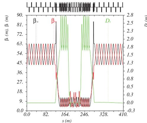
Figure 5: Optics for a preliminary 10 GeV design with an insertion at the centre of the arc and a dispersion suppressor on either side. The suppression of the dispersion can be seen by comparison with Fig. 2.
