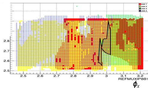
Figure 6: Area of stable phase advance over IR8 that lead to successful optics convergence: For four different scenarios the phase advances are plotted that lead to possible solutions. The black line shows the region where for one common phase all optics conditions can be satisfied.
