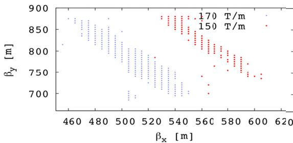
Figure 2: Horizontal and vertical  $\beta$ -functions in front of Q4, which leads to the convergence of the matching. The plot compares the situation of two different triplet gradients.
