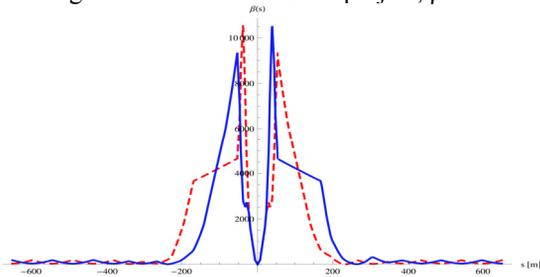
Figure 5: The optics of the long straight section, showing the horizontal (blue) and vertical (red)  $\beta$ -functions as a function of longitudinal distance from IP5, with the matching quadrupoles Q5 and Q6 replaced by doublets.
