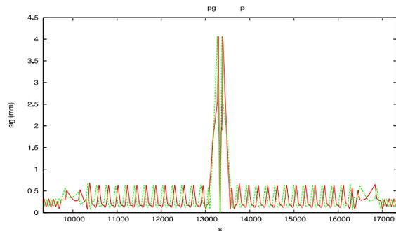
Figure 1: ATS optics with  $\beta^*=10$  cm, at IP5: The transverse beam sizes [mm] are plotted between the neighboring sectors IR4 and IR6.
