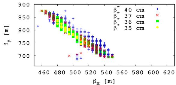
Figure 3: Horizontal and vertical beta functions in front of Q4 which lead to the convergence of the matching of the new triplet (170 T/m) with the LHC lattice in the high luminosity interaction regions.
