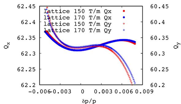
Figure 4: Horizontal and vertical tune for the upgrade optics as a function of  $\Delta p/p$ . The figure compares the situation of two alternative triplet gradients.
