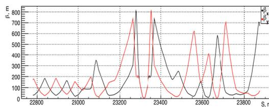
Figure 7: Optical solution for IP8, combining the standard FODO optics (left ) with the ATS optics (right of IP).
