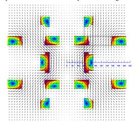
Figure 3: Cross-section of a double half-quadrupole. The coils are wound from simple racetracks in order to facility the production in case Nb<sub>3</sub>Sn superconductor technology would be required.
