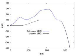
Figure 2: Reference orbit comparison with actual LHC.
