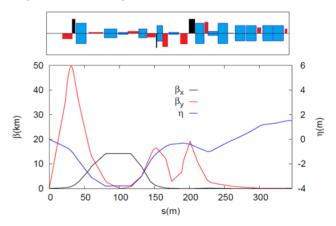
Figure 1: LHC flat-beam IR optics (right side of the IP). Bending magnets are shown in blue, quadrupoles in red and sextupoles in black.
