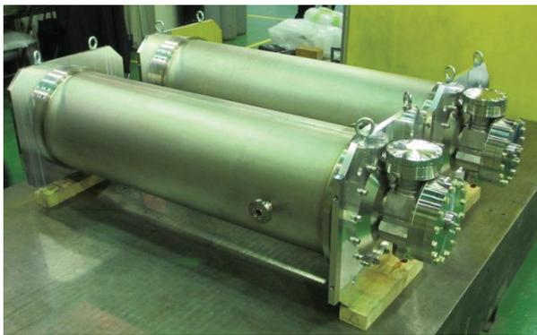
Figure 4: Main linac 9-cell cavities. After the vertical tests, He jackets were welded on them.
