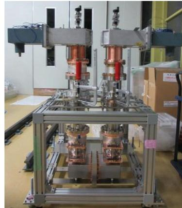
Figure 5: Fabricated input couplers for cERL main linac.
