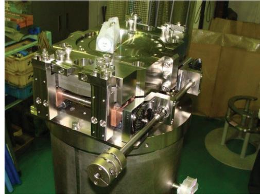
Figure 8: Fabricated frequency tuners for cERL main linac. Tuner is located on the end of the cavity.
