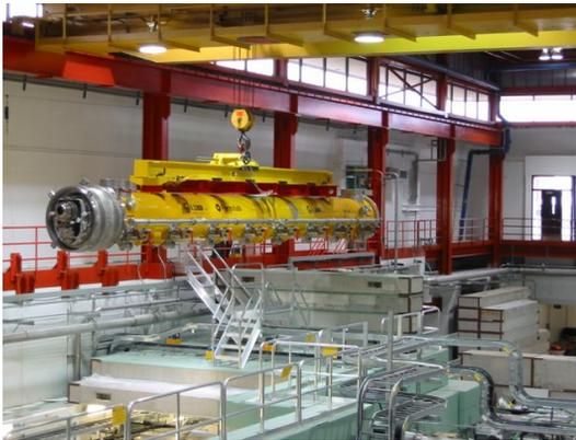
Figure 2: CM1 being removed from ASTA test cave.
