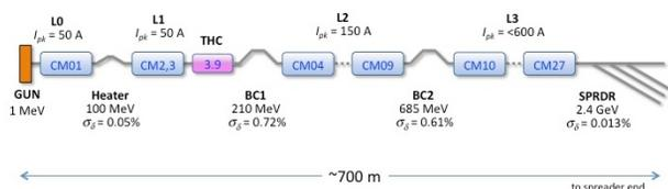
Figure 1: LINAC layout with energies, relative energy spreads ( $\sigma_e$ ) and peak currents.
