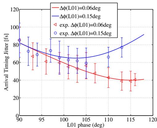
Figure 4: Measurements and theoretical expectation of the ATJ versus linac phase for a RF phase jitter of 0.06 and 0.15 deg S-band.  $R_{56}=-41mm$ ,  $dt_0$  from the injector is 80 fs.
