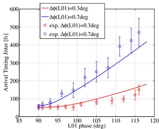
Figure 5: Measurements and theoretical expectation of the ATJ versus linac phase for a RF phase jitter of 0.3 and 0.7 deg S-band.  $R_{56}=-41mm$ ,  $dt_0$  from the injector is 60 fs.
