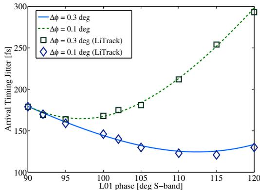
Figure 3:  $dV/V = 0.1\%$ ,  $dB/B = 0.01\%$ ,  $R_{56} = -41mm$ . Initial time jitter:  $150fs$ .
