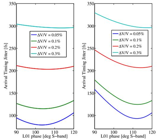
Figure 2:  $d\phi = 0.1deg$ ,  $dB/B = 0.01\%$ ,  $R_{56} = -41mm$ . Initial time jitter  $80fs$  (left) and  $150fs$  (right).
