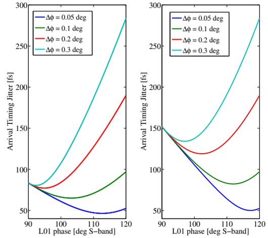
Figure 1:  $dV/V = 0.2\%$ ,  $dB/B = 0.01\%$ ,  $R_{56} = -41mm$ . Initial time jitter  $80fs$  (left) and  $150fs$  (right).
