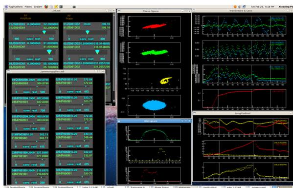
Figure 2: Left: EPICS control sliders. Right: simulation outputs including phase spaces, beam centroids, sizes, emittances, distribution histograms and loss.
