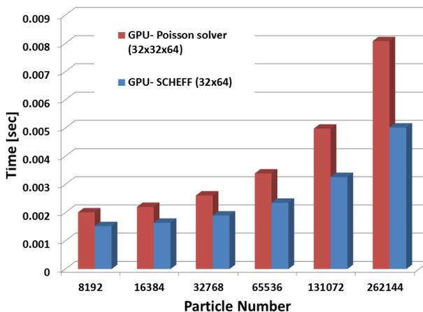
Figure 6: Computing times for 3D Poisson solver and SCHEFF.
