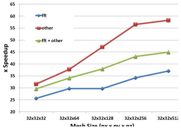
Figure 7: Speedup gained by GPU for 3D Poisson solver.
