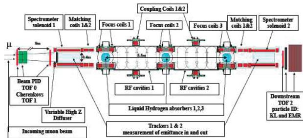
Figure 1: Layout of the muon ionization cooling experiment MICE.
