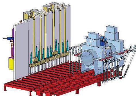
Figure 7: RF power layout in the MICE hall with sketch of one RF module (two are necessary for Step VI).
