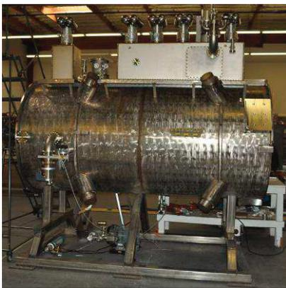
Figure 5: Completed spectrometer solenoid at Wang NMR, Inc. of Livermore, CA.
