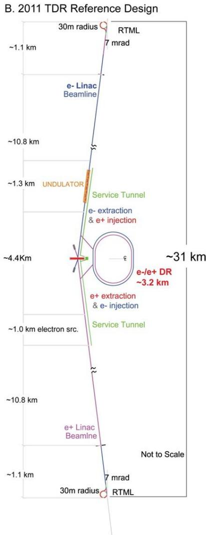
Figure 3: The ILC general lay-out.
