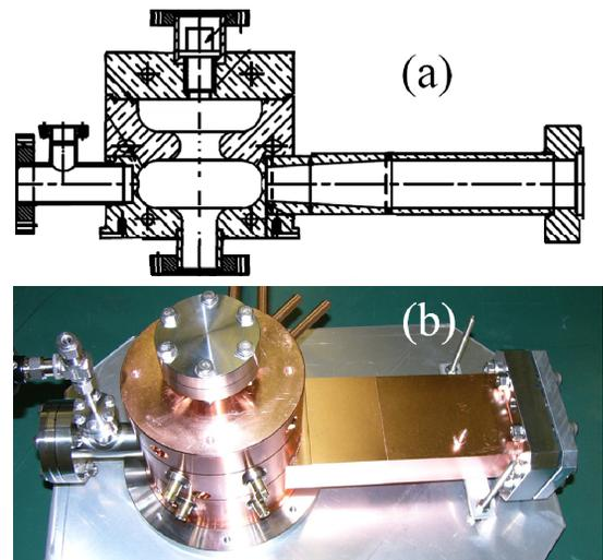
Figure 5: New femtosecond photocathode rf gun for ultrafast electron diffraction and microscopy.
