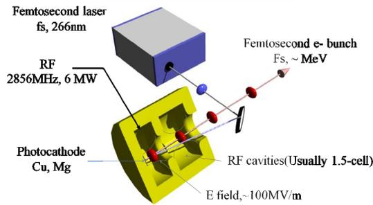
Figure 1: Concept of femtosecond photocathode RF gun.
