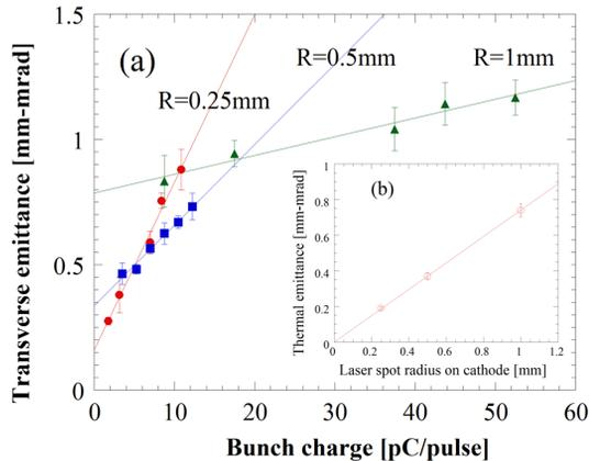
Figure 3: (a) transverse emittance as a function of bunch charge, (b) thermal emittance as a function of laser spot radius on the copper cathode.
