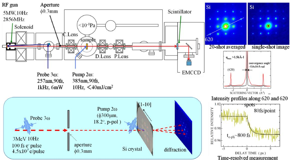
Figure 6: RF gun based UED facility at Osaka University and the experimental results in single-crystal Si: a 20-shot averaged image, a single-shot image, intensity profiles, and ultrafast dynamics observed by time-resolved measurement.
