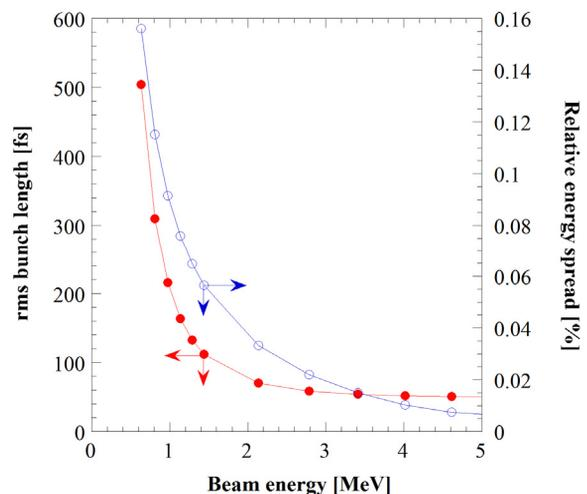
Figure 2: Simulation results of bunch length and energy spread as function of beam energy in the RF gun at the bunch charge of 0.1 pC.
