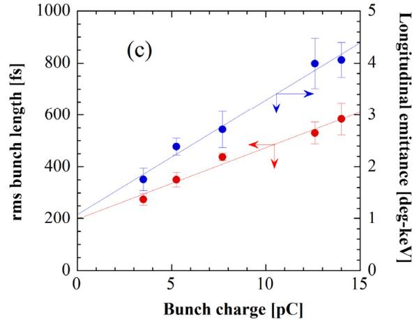
Figure 4: Bunch length and longitudinal emittance measured as a function of bunch charge.
