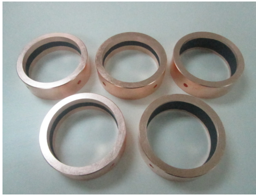
Figure 5: Five FeSiAl collinear load cavities ring.
