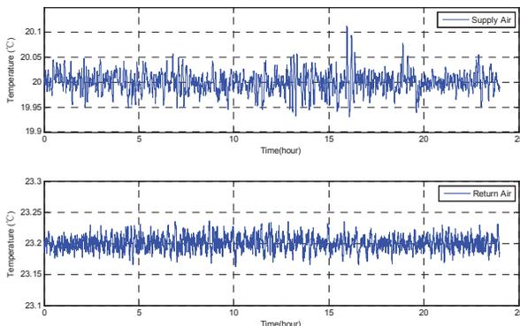
Figure 5: Highly precise control of temperature with run-around coils.
