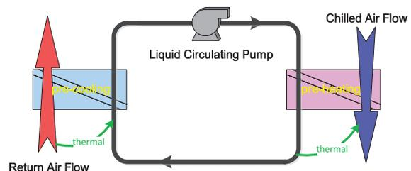
Figure 1: Scheme of run-around system to recover heat and moisture.
