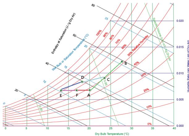
Figure 3: Psychrometric diagram of HVAC commissioning with run-around coils.
