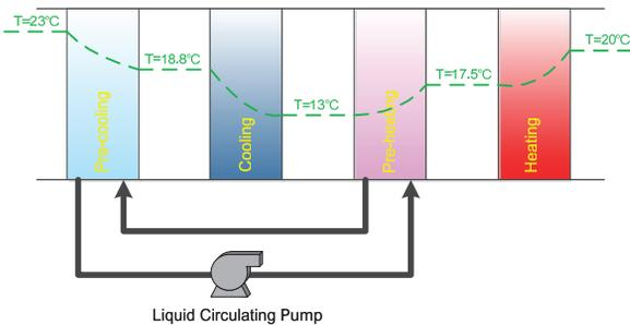
Figure 2: Proposed AHU with run-around coils.
