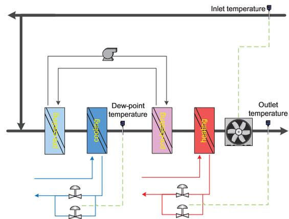
Figure 6: Block diagram of the control philosophy.
