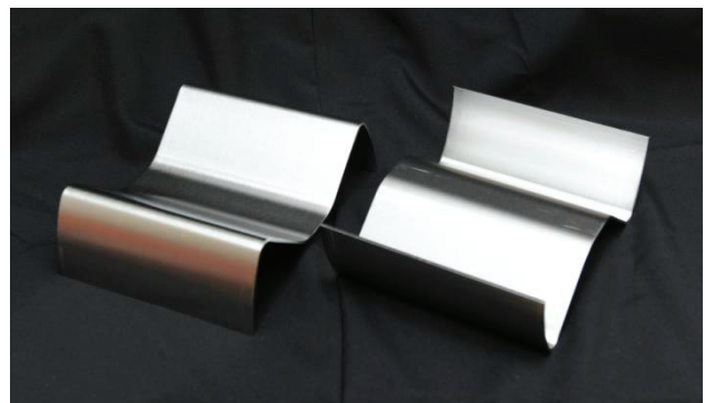
Figure 5: Half shells before welding
