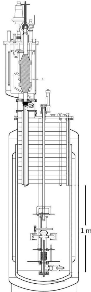
Figure 1: Test cryostat layout.
