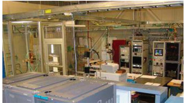
Figure 4: SPX rf test stand area showing clean room for waveguide and damper particulate testing on the left and 4-kW rf system on the right.
