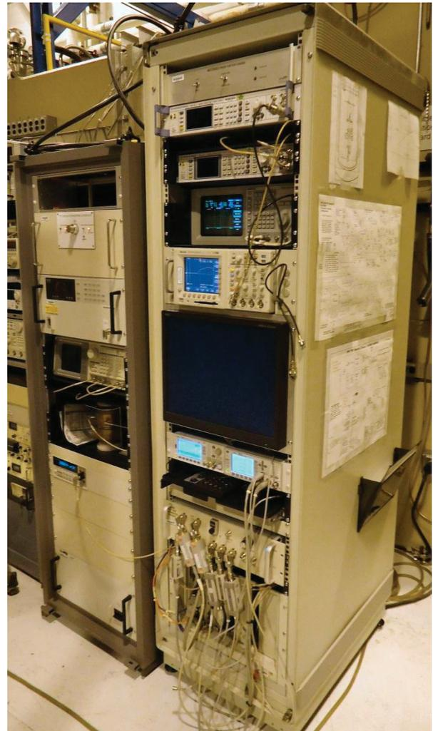
Figure 5: SPX rf test stand for vertical cavity testing at the ATLAS SRF Cavity Test Facility.
