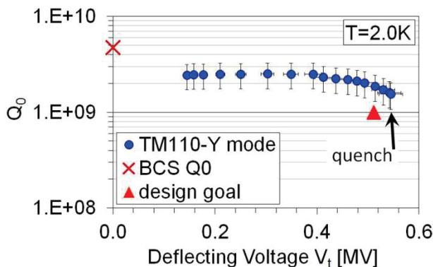
Figure 6: Cavity Q vs. deflecting voltage at 2.0 K
