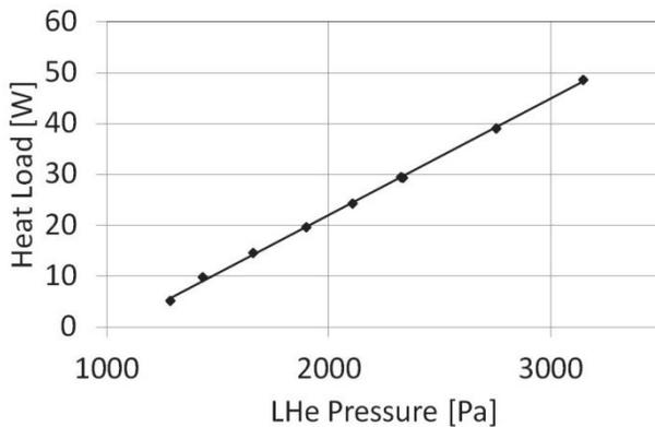
Figure 3: Cryostat vacuum system performance.
