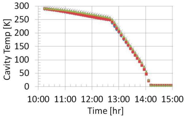
Figure 2: Cavity cooldown in the test cryostat.
