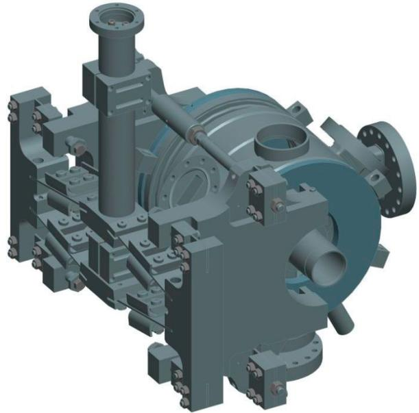
Figure 7: Dressed SPX cavity showing titanium helium tank, coupling ports, and mechanical slow tuner.
