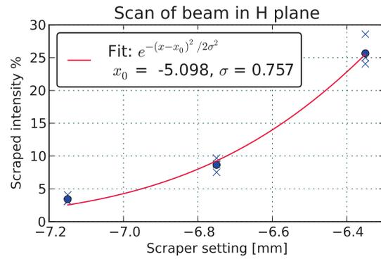
Figure 8: The horizontal scan was repeated after 1.5 hours using three measurement points. The obtained beam position is similar to the result in Fig. 6.
