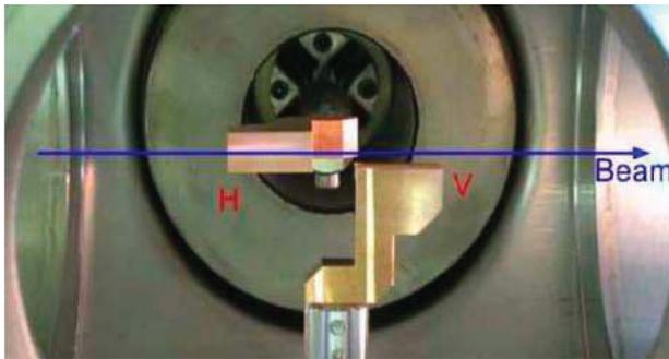
Figure 1: Picture of a copper scraper installed in the SPS. Courtesy of H. Burkhardt.
