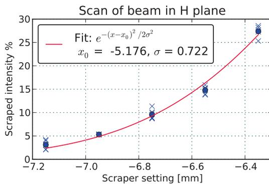
Figure 6: Horizontal scraper scan: The beam size and position are calculated by fitting Eq.1.
