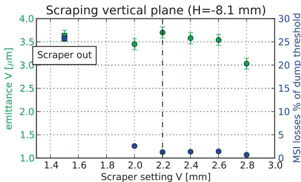
Figure 5: Measured emittance in the vertical plane and losses at the MSI versus vertical scraper position for initially nominal emittance beam ( $3.5 \mu\text{m}$ ). The horizontal scraper was kept constant at -8.1 mm. Losses are reduced from 25.8% (no scraping) to 1.3% of dump thresholds with the scrapers at nominal setting. Moving the scraper further into the beam does not significantly reduce the losses further.
