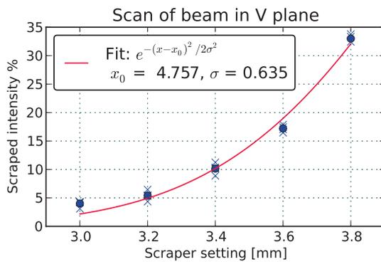
Figure 7: Vertical scraper scan: The beam size and position relative to the scraper are calculated using Eq. 1.
