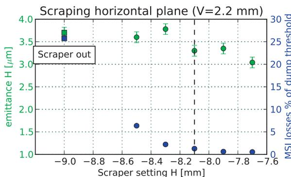
Figure 4: Measured emittance in the horizontal plane and losses at the MSI versus horizontal scraper position for initially nominal emittance beam ( $3.5 \mu\text{m}$ ). The vertical scraper was kept constant at 2.2 mm. The losses could be reduced from 25.7% (no scraping) to 1.3% of dump threshold without reducing the emittance. Moving the scraper further into the beam does not significantly reduce the losses further.
