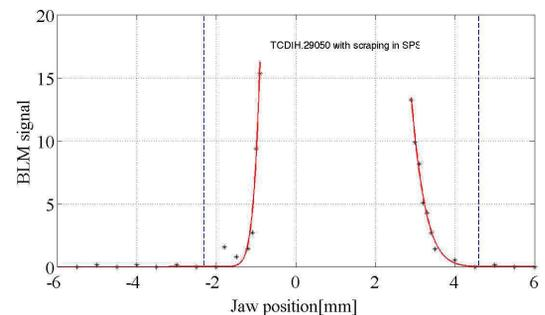
Figure 3: Tail scan at horizontal transfer line collimator (TCDIH.29050) after scraping: Scraping removes the particles in the tails. The number of particles impacting the collimator is much reduced. (Nominal collimator position in blue).
