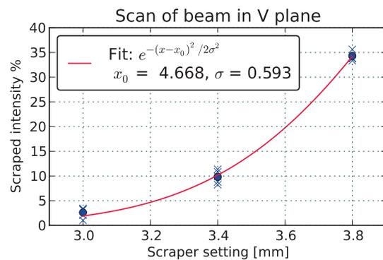
Figure 9: After about 1.5 hours the vertical scan was repeated using three measurement points. The beam position is similar to the result in Fig. 7.
