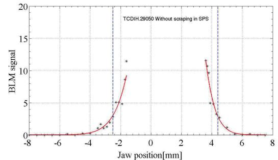
Figure 2: Tail scan at horizontal transfer line collimator (TCDIH.29050): The nominal collimator position is marked with blue lines. Without scraping the tails of the beam distribution impact the collimators.
