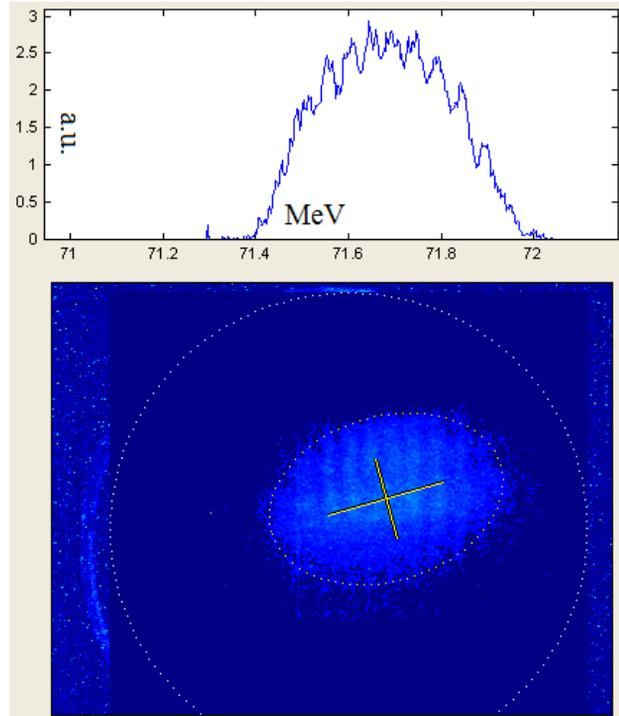
Figure 2: Zero phasing measurement of the 90 pC, 3 ps (FWHM) long electron beam produced by the longitudinally modulated photocathode laser. The wavelength of the induced modulation is 60  $\mu\text{m}$ .
