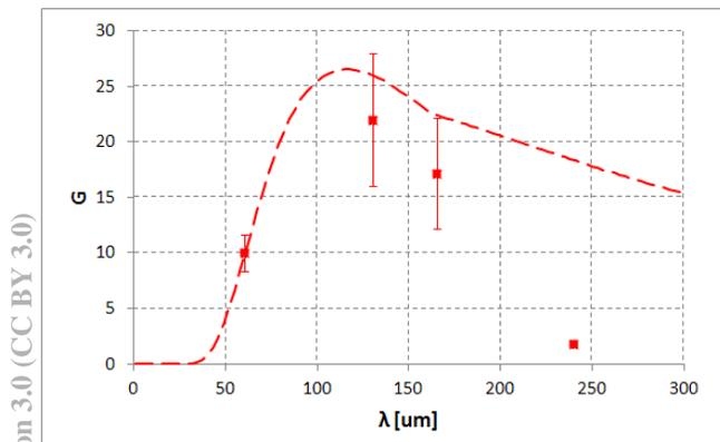
Figure 4: Comparison of the direct measurement of microbunching gain (dots) and the theoretical predictions (line). Horizontal axis shows modulation wavelength of the uncompressed beam. The vertical axis shows microbunching gain.
