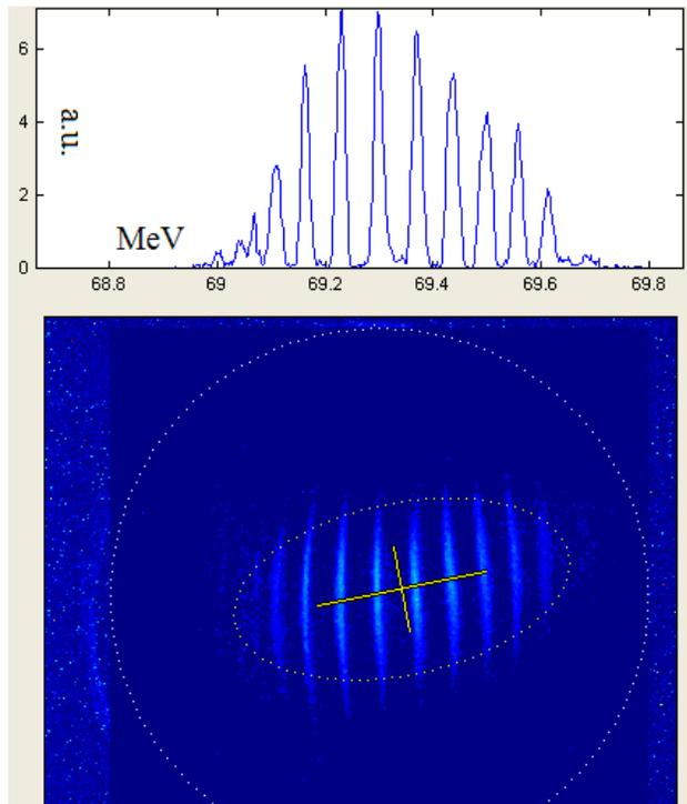
Figure 3: The zero phasing of the compressed 90 pC beam. The BC compression factor is 2.5.
