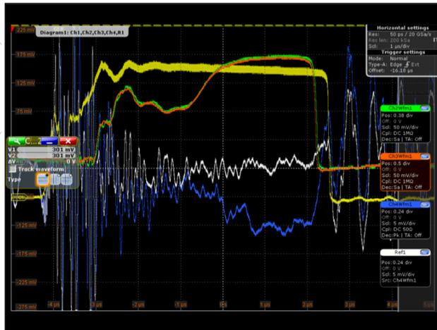
Figure 4: Observation of spontaneous emission with a mercury cadmium telluride (MCT) detector – blue trace.
