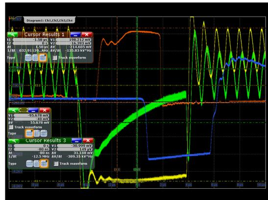
Figure 6: Blue MCT detector signal confirming first light.
