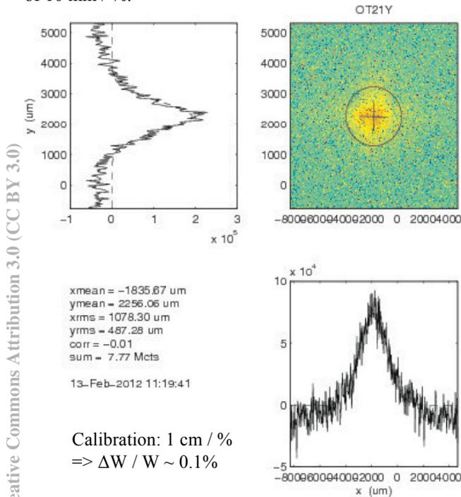
Figure 3: Measurement of 0.1% energy spread at 25 MeV.
