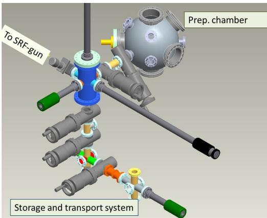
Figure 6: contracture design of new GaAs preparation system.
