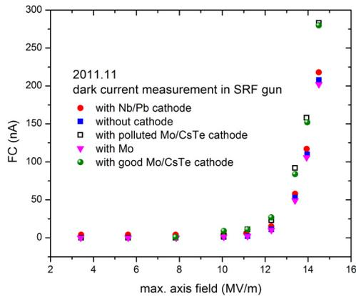
Figure 2: Dark current measurement with different cathode material.
