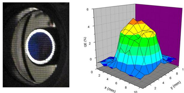
Figure 1: Cathode #250310Mo in vacuum and QE distribution map. It was in gun from 2010.5.25 to 2011.7.26. Total beam time was over 1000 h, and extracted charge was about 35 C.
