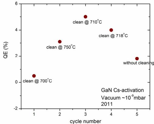
Figure 5: The first series GaN activation tests have been performed on  $10^{17}$ -level p-doped GaN grown on sapphire. The samples could be reactivated several cycles.
