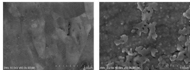
Figure 4: SEM-morphology: (left) optical-polished Mo substratum; (right) Cs/Sb film deposited with rate 2.7 on Mo substratum.
