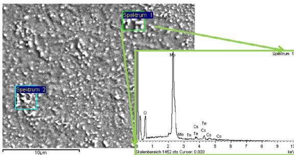
Figure 3: SEM/EDX analysis for Cs<sub>2</sub>Te photocathode #060410Mo. Spectrum shows the element content (Cs/Te=2.3) in the center of film.
